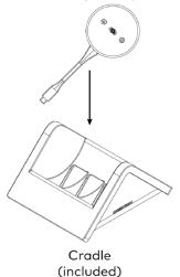
Connect up to two cradles to store additional AM-TX3-100 adaptors. The cradles connect end-to-end using integrated magnets.
